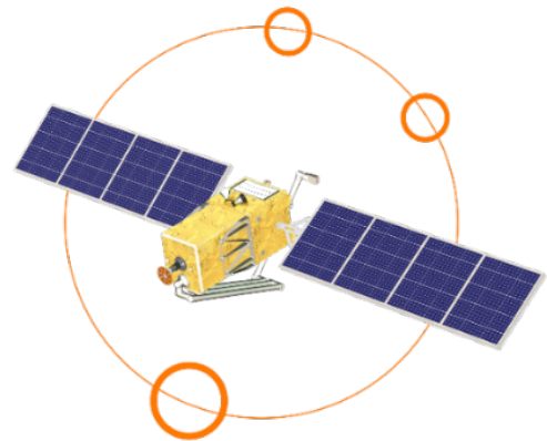
Figure 1: Diagram of the Otter satellite servicer: a low-SWaP spacecraft designed for autonomous capture and maneuver of free-flying objects. Otter features CEPHALOPOD autonomous trajectory generation and, CETACEAN relative navigation software, and Nautilus non-destructive capture mechanism, a hardware solution that does not require pre-configured docking
