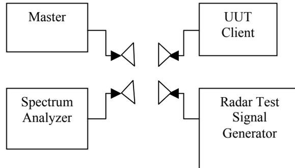
**Set-up C: Client with injection at the Client**
