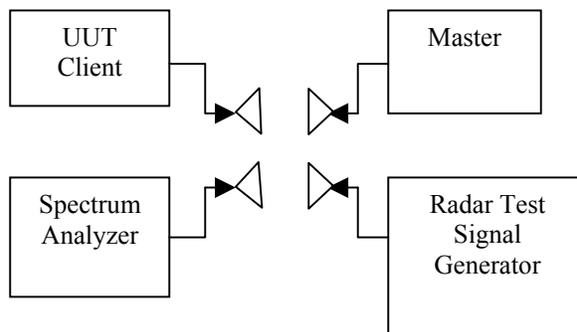
For the purposes of the test, the UUT as well as other unlicensed U-NII devices used in the set-up may be equipped with a specific user interface to allow monitoring of the behavior of the different devices of the set-up during the tests.
