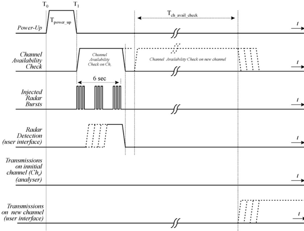
***Radar burst at the end of the Channel Availability Check Time***
