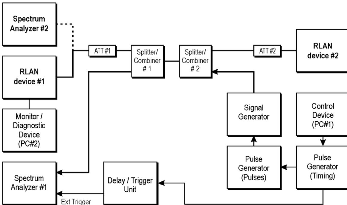
It is important to note that the Signal Generator used should have the 'Short Pulse' option to guarantee that the Automatic Level Control circuitry can also deal with short pulses (this will be verified during the calibration part.). It might be possible that the function of the Delay/Trigger unit is part of the features of Spectrum Analyzer #1.
