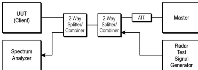
For the purposes of the test, the UUT as well as other unlicensed U-NII devices used in the set-up may be equipped with a specific user interface to allow monitoring of the behavior of
